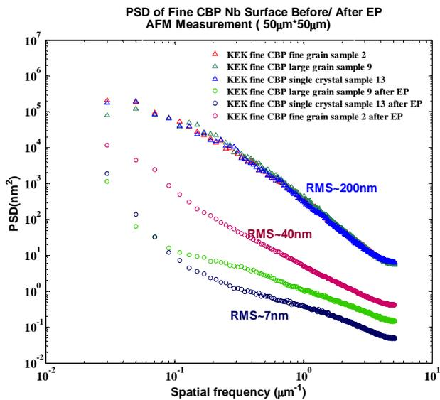
Figure 5: The PSD of fine CBP polycrystalline, large gain and single crystal Nb samples after 30 µm removal by EP at 30±1°C.
