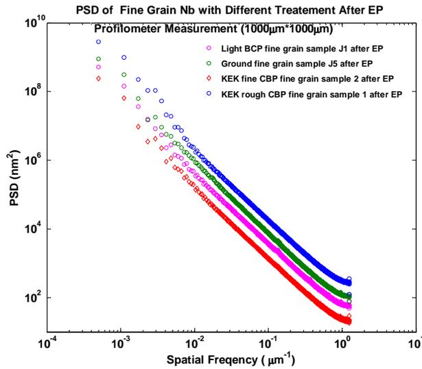
Figure 4: The PSD of rough CBP, fine CBP, hand grinding and light BCP treated polycrystalline Nb sample after 30µm removal by EP at 30±1°C.
