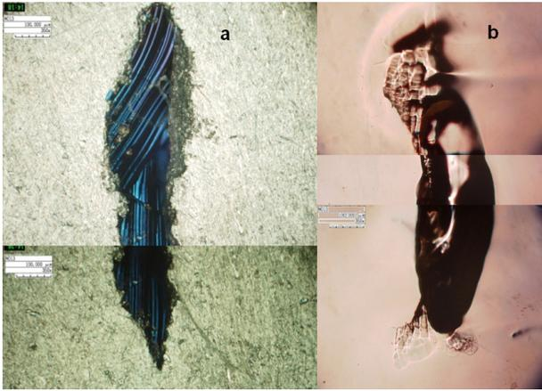
Figure 1: The optical microcopy image of a defect on the fine CBP EBW single crystal Nb sample (KEK-17) before and after EP.
