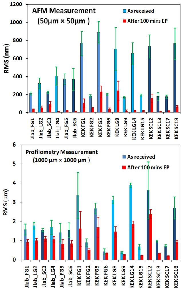
Figure 2: The statistical results of AFM (above) and SP measurements (below) for 24 samples studied before and after EP.
