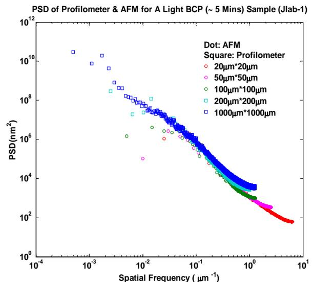
Figure 3: Combined AFM and profilometer power spectral densities from all scan sizes from the sample having undergone 5 minutes of BCP treatment.
