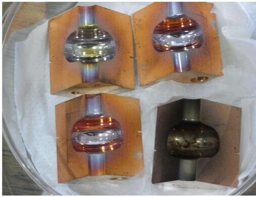
Figure 5: Four annealed quadrant. The upper left one became superconductive.
