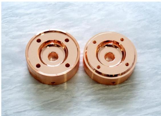
Figure 2: Two parts machined vertical to the axis are assembled to make a cavity. The inside surface is to be covered with  $\text{MgB}_2$  films.
