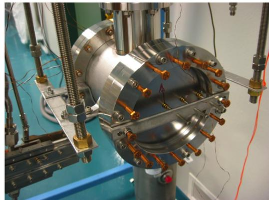
Figure 7: Niobium test chamber. The temperature sensors shown are for direct measurement of temperature increase due to the heater placed on the other side of the 2 mm thick Nb plate.
