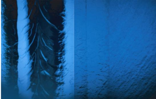
Figure 7: Image of the RF surface at equator region of A12 near quench site. No unusual feature is observable despite the appearance of a quench-correlated hot spot by T-mapping. The quench field was raised from 32 MV/m to 40 MV/m by a light EP processing of 25  $\mu\text{m}$ .
