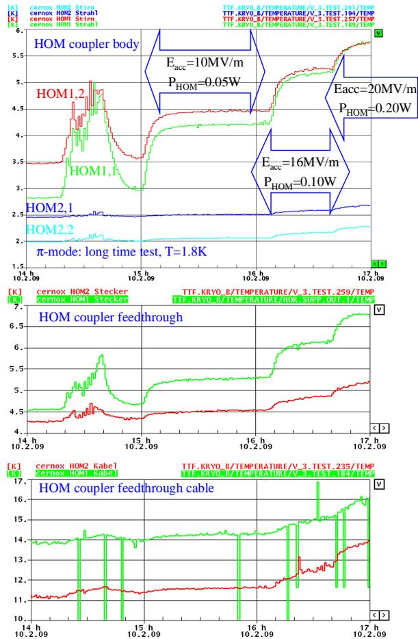
Figure 9: Cavity AC128 long time test history: HOM couplers temperatures (feedthroughs are connected to 2 K cooling circle).
