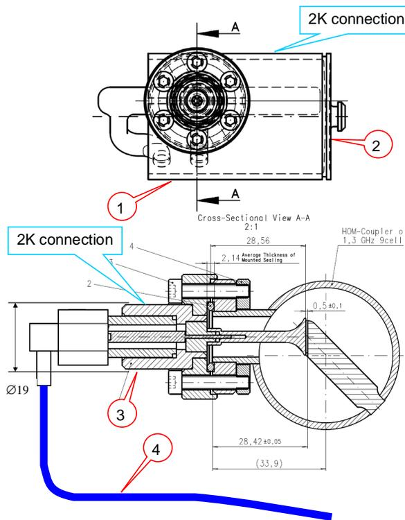
Figure 3: HOM coupler with a new feedthrough (JLAB design), with temperature sensors positions.
