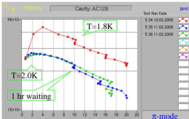
Figure 8: Cavity AC128 horizontal tests: long time test history.
