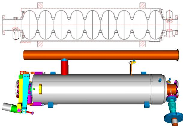
Figure 1: SRF cavity in LHe tank with auxiliaries.
