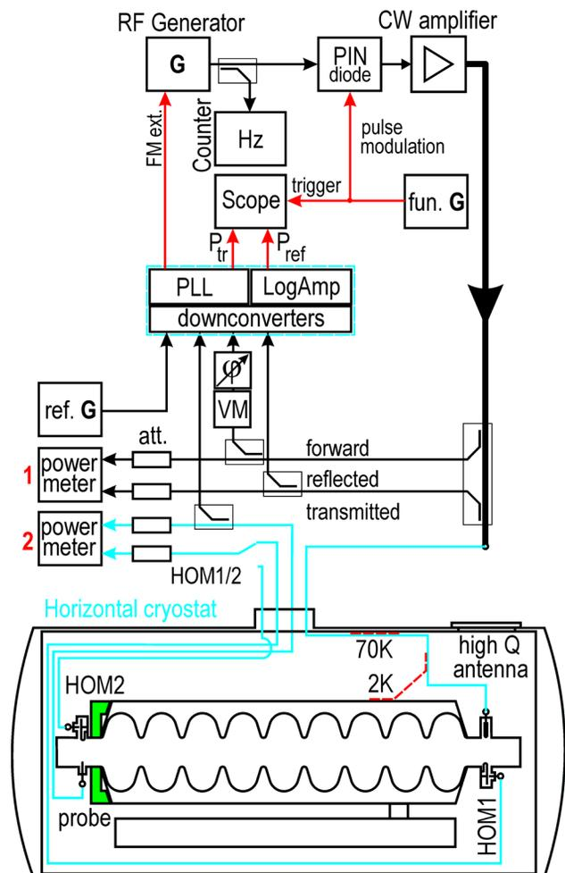
Figure 2: Superconducting cavity CW test in horizontal test cryostat.
