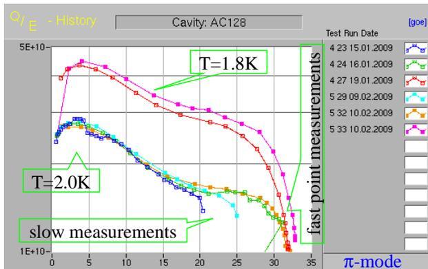
Figure 7: Cavity AC128 horizontal tests: cavity performance improvement with connection of HOM coupler feedthroughs to 2K.
