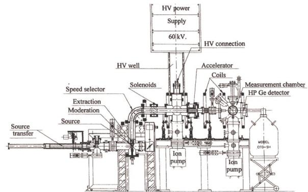
Figure 4: Schematic view of slow positron beam facility in Orléans [12].
