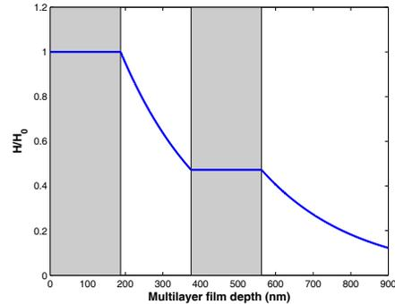
Figure 1: As in [1], the normalized field  $H/H_0$  as a function of sample depth for alternating layers of Nb-Ti and  $\text{Al}_2\text{O}_3$ .  $\lambda \sim 250$  nm and the layer thickness  $d \sim 0.75\lambda$ .
