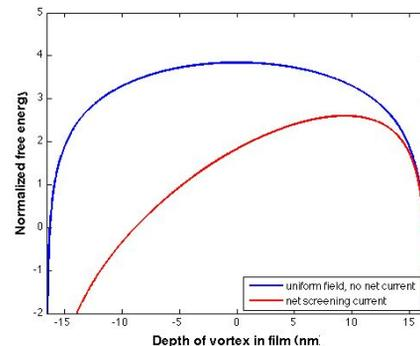
Figure 2: As in [1], the normalized vortex free energy  $G/G_0$  as a function of displacement  $u$  from the center of a superconducting Nb-Ti film. The red line represents the barrier to flux motion arising from a net current across the film.
