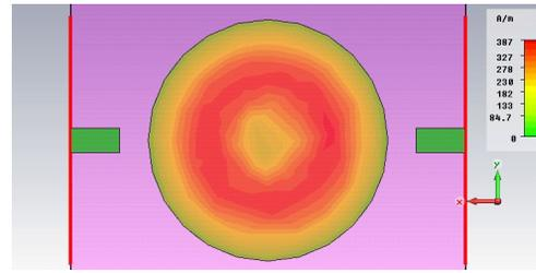
Figure 3: CST Microwave Studio finite element simulation of the magnetic field from a microstrip disk resonator. The field is entirely tangential to the disk surface, with no radial or longitudinal components. Stripline for capacitive RF coupling is seen on either side of the disk.
