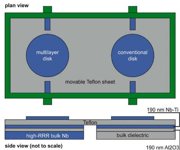
Figure 4: Schematic of the experimental apparatus. Multilayer and “control” samples are deposited simultaneously on the same substrate.
