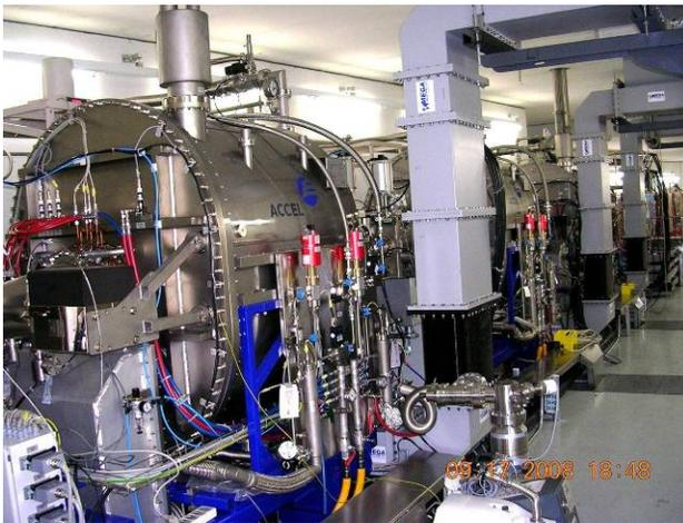
Figure 2: SRF modules in the tunnel of storage ring.
