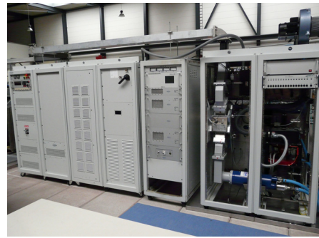
Figure 9: Test setup of the 30 kW IOT amplifier at ELBE.
