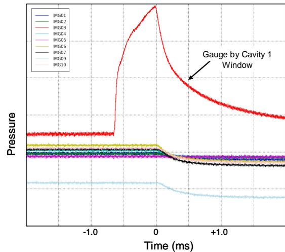
Figure 3: Plot of vacuum data during a beam conditioning trip. Here the only signal is on the window of Cavity 1 as the gas cannot propagate through the cold waveguide bend.
