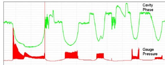
Figure 5: Plot of gauge pressure in the waveguide/window as the phase of the cavity is changed.
