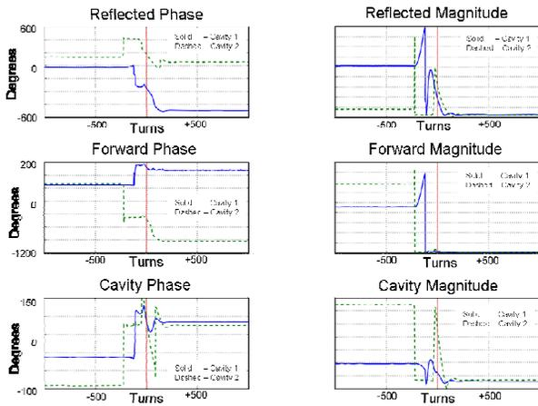
Figure 1: Plot from the RF post-mortem. This shows the magnitude and phase of the forward and reflected power and cavity field relative to the MPS trigger at t=0.
