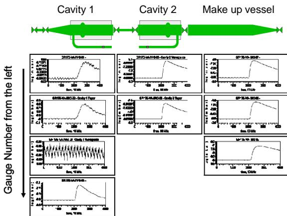
Figure 2: Vacuum signals following an RF trip.
