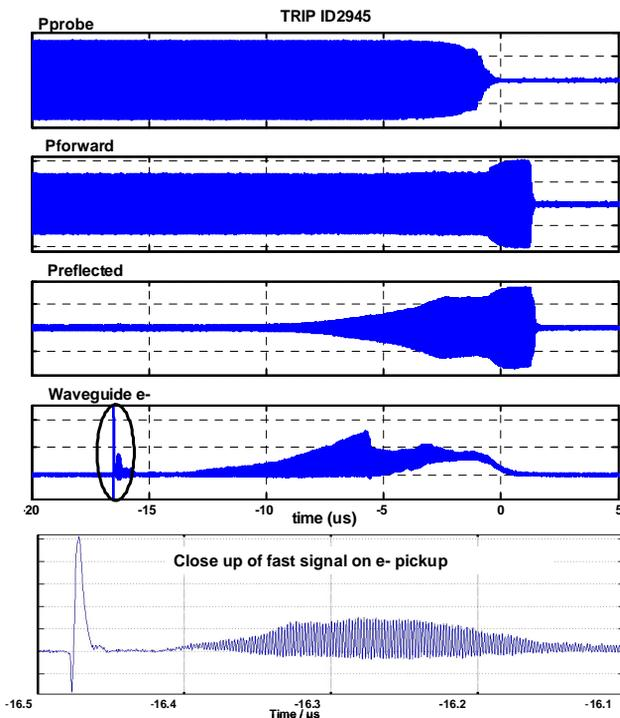
Figure 4: Plot of signals measured immediately before and after a cavity trip. The top 4 plots show 25  $\mu\text{s}$  worth of data and the bottom plot shows a close up of the region circled on the waveguide e- pickup.
