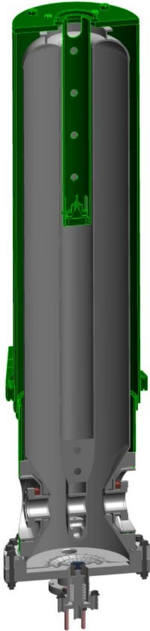
Figure 1. Isometric sectional view of the  $\beta_m = 0.041$  QWR with its helium vessel, stiffening elements, frictional damper, tuning plate, and bottom flange. The helium vessel and damper are shown in green.
