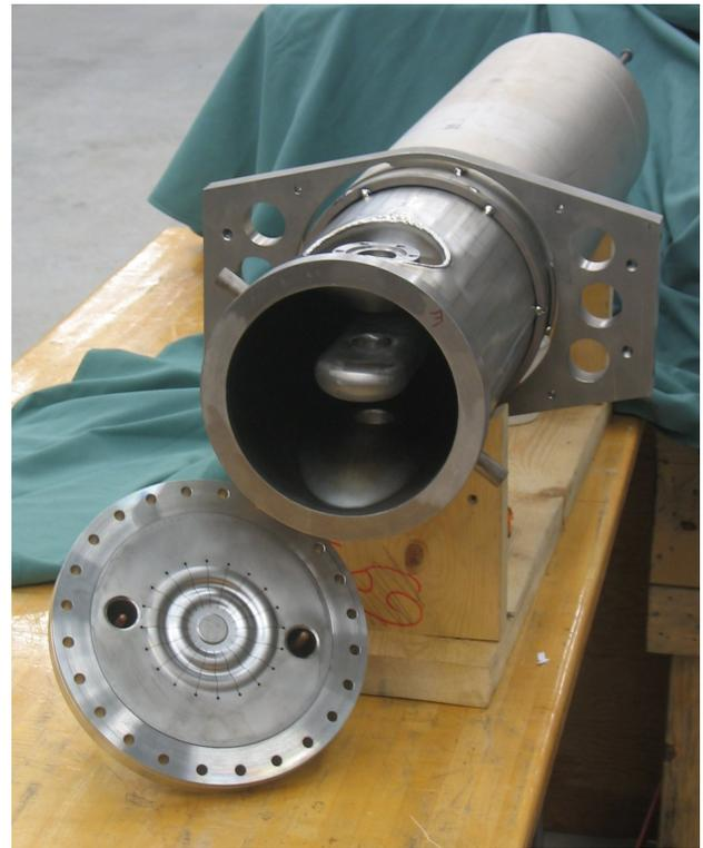
Figure 2. Photograph of a  $\beta_m = 0.041$  QWR after tack welding of the helium vessel. The support flange is welded to the helium vessel. The niobium tuning plate and stainless steel bottom flange are visible on the lower left-hand corner.
