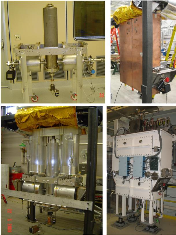
Figure 6. Construction of the rebuncher cryomodule. Top left: cold mass in the clean room; Bottom left: cold mass under top plate; Top right: 77 K shield; Bottom right: completed cryomodule after installation on the ReA3 deck.
