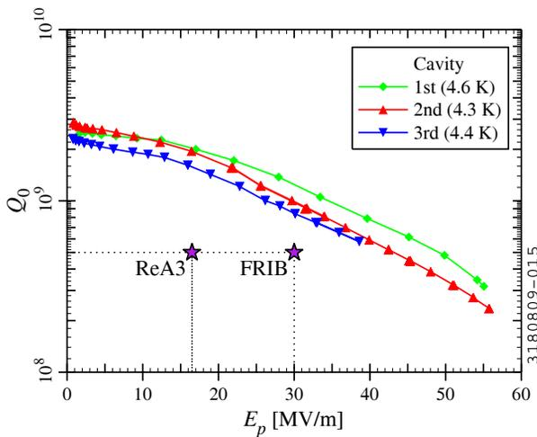
Figure 4. Dewar test results for the first three  $\beta_m = 0.041$  QWRs. The tests on the second and third cavities were done after the installation of the helium vessel.
