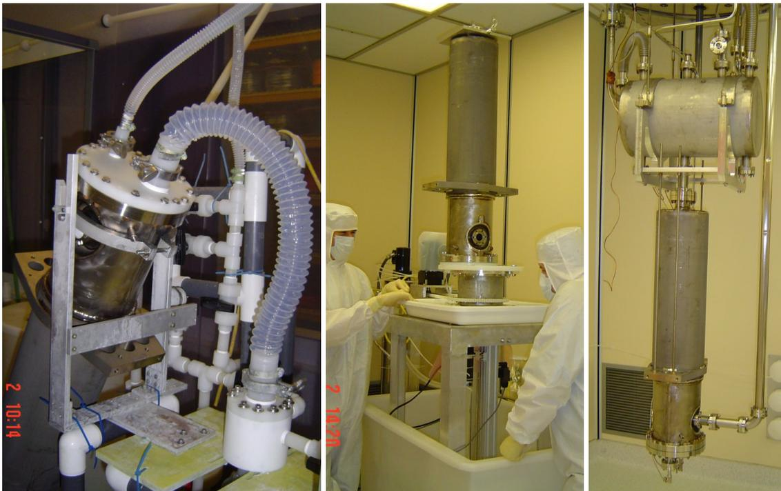
Figure 3. Left to right: etching, rinsing, and assembly of a  $\beta_m = 0.041$  QWR onto the insert for Dewar testing.
