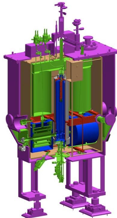
Figure 5. Isometric sectional view of the rebuncher cryomodule.
