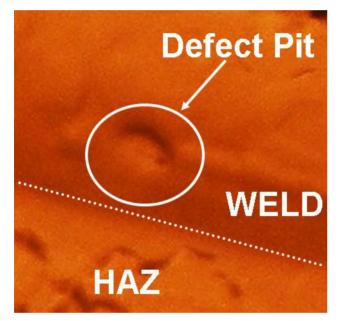
Figure 2: The 9-cell reentrant cavity pit defect.
