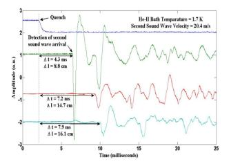
Figure 1: A quench event. Four traces are shown: 1) the upper trace is the quenching-cavity transmitted power, 2-4) the lower traces are transducer second sound signals.
