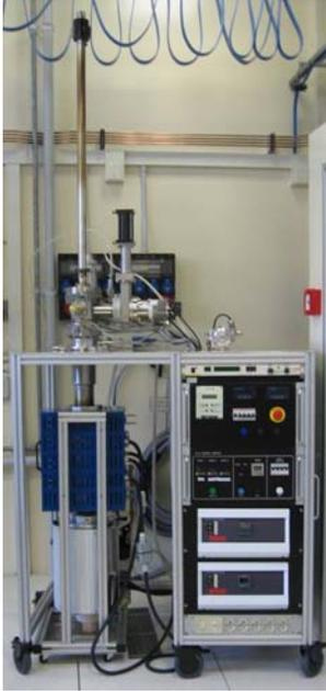
Figure 2: Our “Double Furnace System”. It was built to simplify the experimental procedure. Now it is possible to perform the annealing in vacuum without opening the chamber to remove the Sn crucible.
