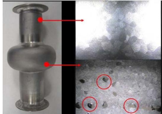
Figure 4:  $Nb_3Sn$  6 GHz cavity obtained using the “double process”. The unreacted Sn problem is still present.
