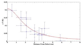
Figure 3: An example of the spatial distribution of cavity heating due to a defect.
