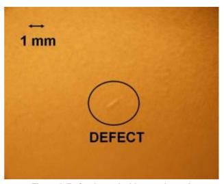
Figure 5: Defect located with second sound.
