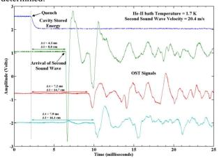
Figure 2: A typical quench event observed with three different transducers. The top trace is the amplitude of the cavity RF field. The lower three traces are the second sound signals measured with 3 distinct OST. The variation in the second sound wave time-of-arrival is well correlated with the variation in propagation distance to each transducer.
