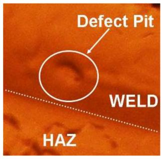
Figure 6: Defect located with second sound on a cavity equator weld. The defect is circles and the weld and heat affected zone (HAZ) are labeled [9].
