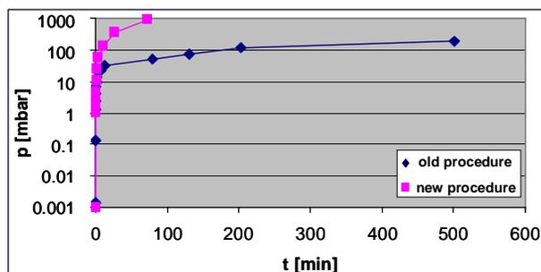
Figure 3: Pressure versus time during venting of a cavity string using the old procedure (◆) and new procedure (■).
