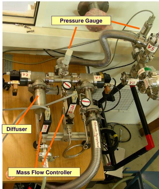
Figure 1: Improved set-up for particle free pump down and venting: schematics (left) and photograph (right).
