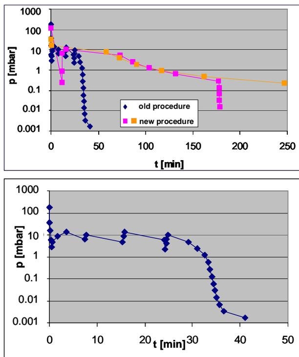
Figure 2: Pressure versus time during pump out of a cavity string using the old procedure (◆) and new procedure (■, □). The lower graph shows the old procedure with an enlarged time scale.
