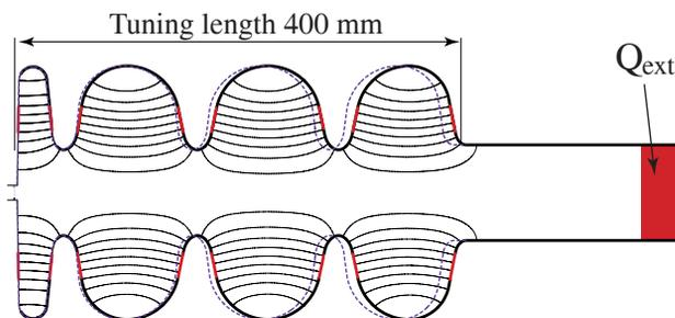
Figure 1: The 3½ cell cavity of FZD like SRF gun. The detuning cavity length principle is demonstrated.
