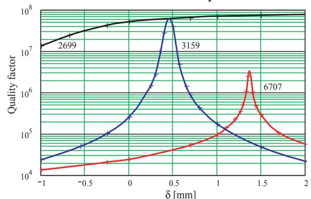
Figure 2: Trapped dipole HOM external quality factor versus the cavity longitudinal deformation.
