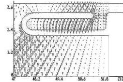
Figure 7: The electric dipole field distribution in the dipole notch filter (CLANS2 output).
