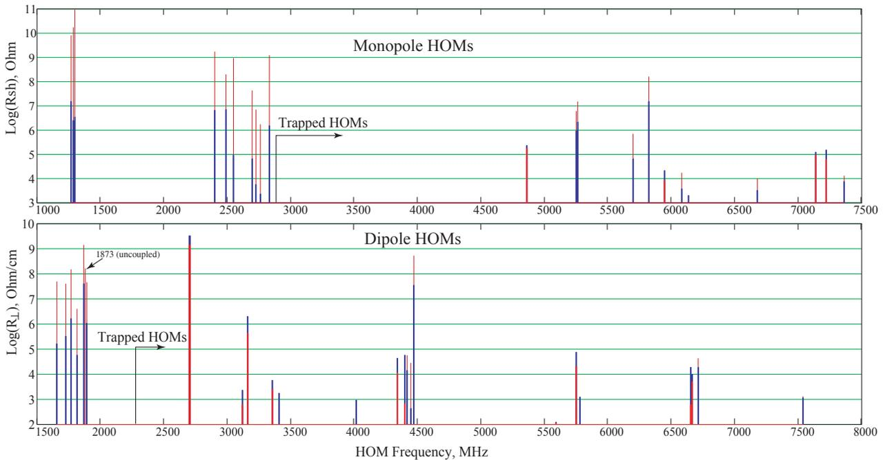
Figure 4: Monopole [3] and dipole spectrums in the RF gun cavity: red - without the insert (see Fig.1), blue - with the insert that is shown in Figs. 5, 6.
