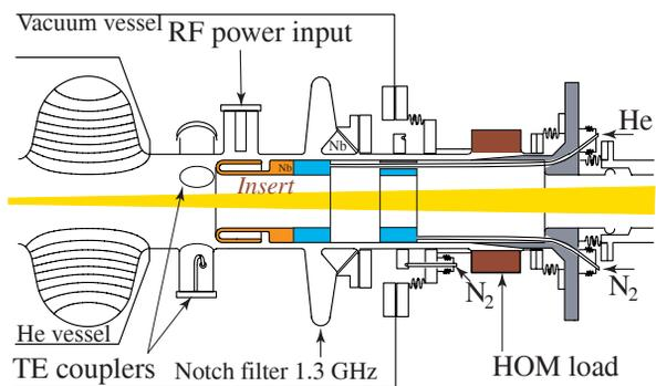
Figure 6: The second variant of HOM damping with superconductive insert, conventional RF power input, and the notch inside the cryostat.
