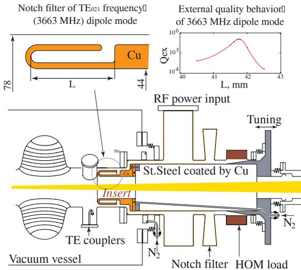
Figure 5: First variant of HOM damping with RF power input and the notch outside the cryostat.
