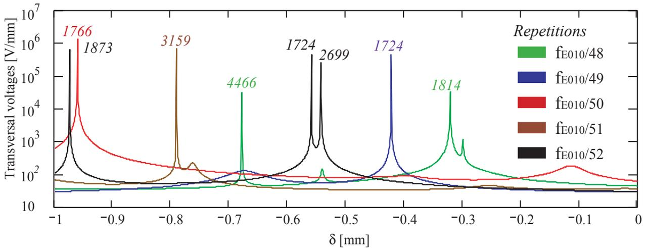
Figure 3: Transversal voltage of all dipole HOMs excited by a 2 mA beam of different repetition frequencies versus the cavity detuning ( $\delta$  parameter).
