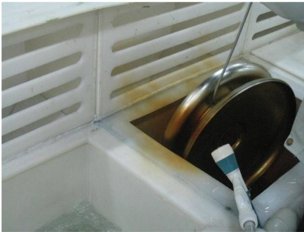
Figure 6: Etching before the electron beam welding.
