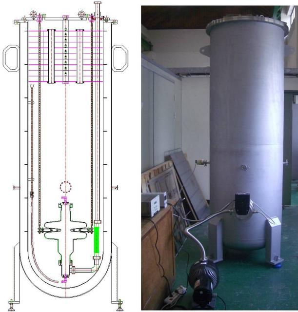
Figure 14: Cryostat for the vertical test.
