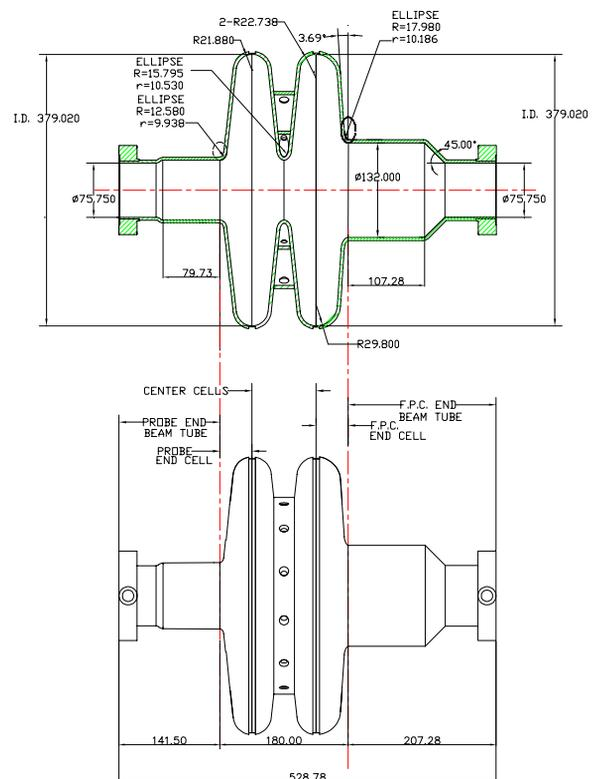
Figure 1: Drawing of the two-cell cavity.
