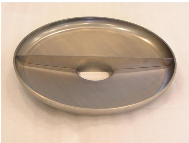
Figure 3: Half-cell after deep drawing.
