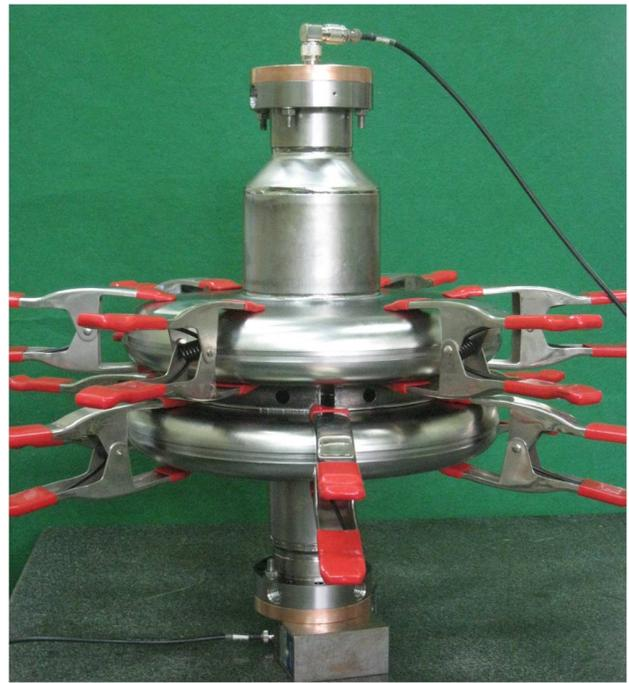
Figure 8: Frequency measurement set-up.
