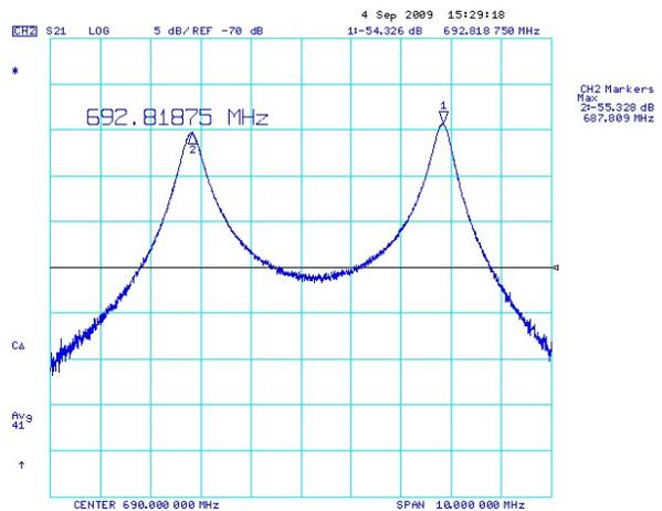
Figure 9: Frequency spectrum before equator welding.
