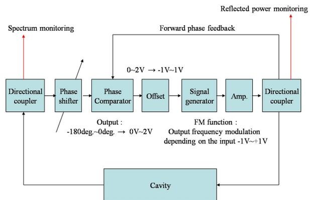
Figure 13: RF System setup for the vertical test.
