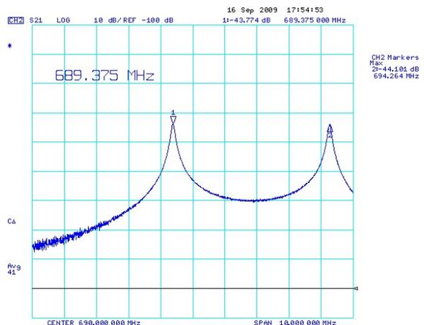
Figure 10: Frequency spectrum after equator welding.
