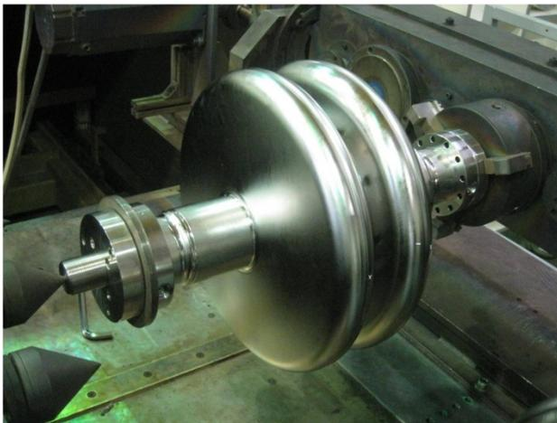
Figure 7: Cavity mounted on the electron beam welder.
