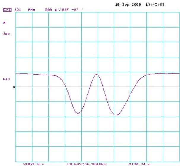
Figure 12: Phase shift during bead-pull test.
