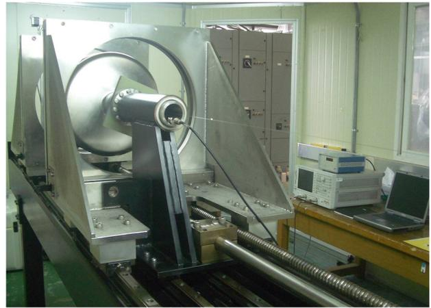
Figure 11: Bead-pull test to measure the field flatness.
