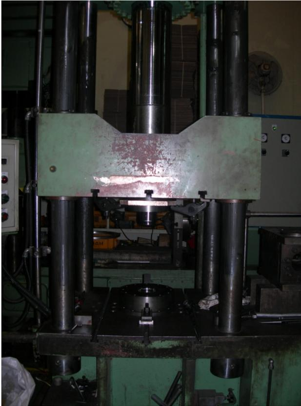
Figure 2: Deep drawing process to make a half-cell.
