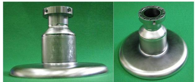
Figure 5: End cell sub-assembly. Left: FPC beam tube, Right: Field probe beam tube.
