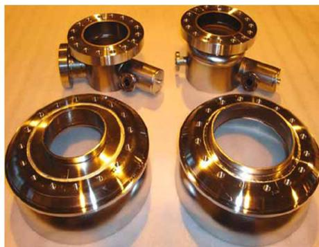
Figure 7: The welded base-plate on end group.
