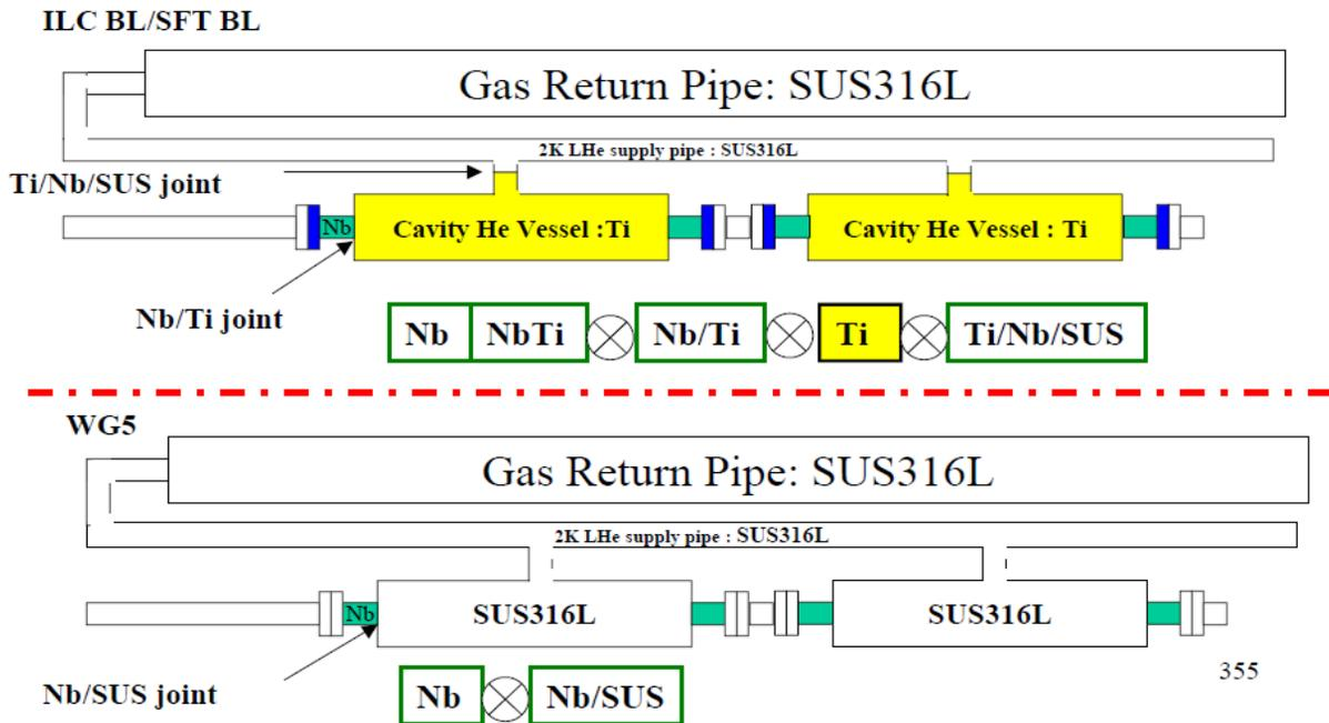
Figure 2: Materials for cryomodule integration.
