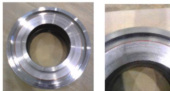
Figure 4: A machined roughly helium base-plate (left). The picture zoomed around the insulated copper area (right).
