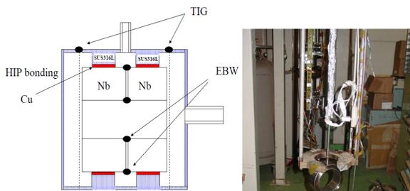
Figure 6: An example of cold leak tested base-plates. The left is welded pieces; the right after TIG welded pieces on the cold leak test line.
