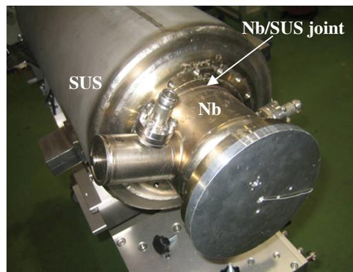
Figure 8: The cavity dressed helium vessel.
