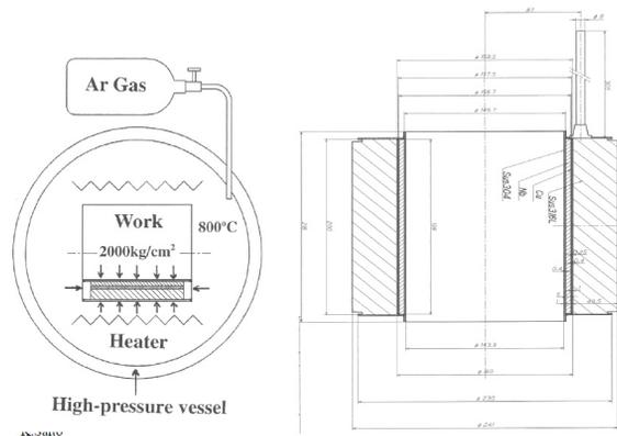
Figure 3: HIP bonding method.
