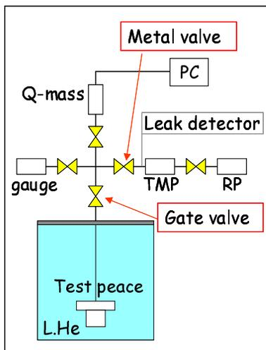
Figure 5: High sensitive cold leak test system at KEK.
