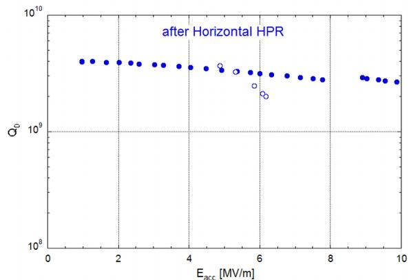
Figure 5:  $Q$ - $E_{acc}$  curve measured after HHPR
