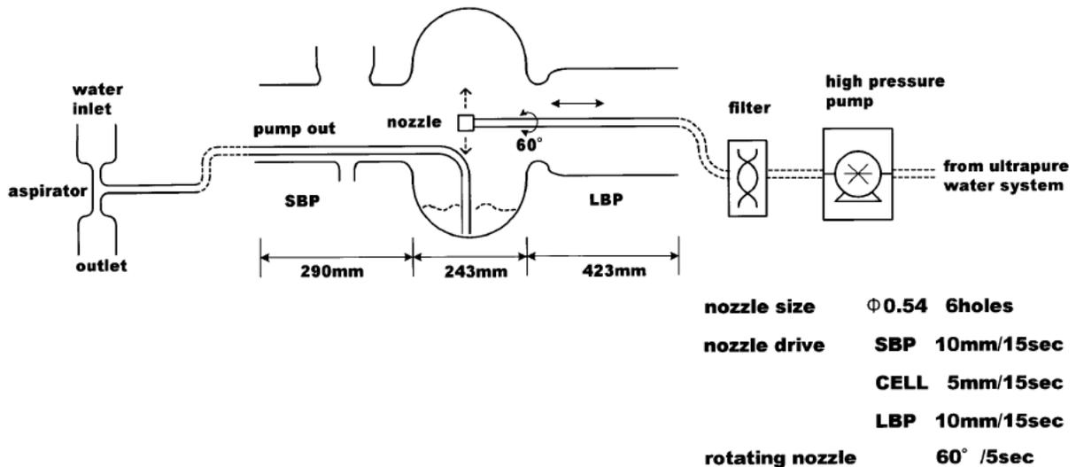
Figure 1: Conceptual design of horizontal high pressure water rinsing system.
