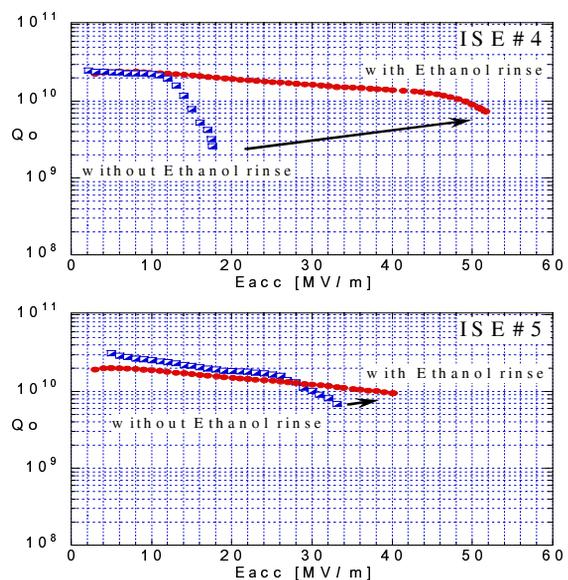
Figure 2: Improvement by ethanol rinsing, Top: ISE#4, Bottom: ISE#5
