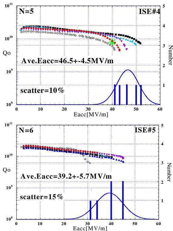
Figure 3: Series test of ethanol rinsing. Top: ISE#4, Bottom: ISE#5
