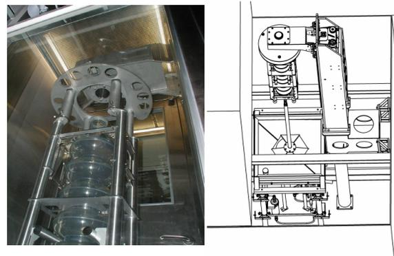
Figure 3: Left: View on the cavity adapter lever arm. Right: Schematic of the HPR system with lever arm motion unit and cavity installed.
