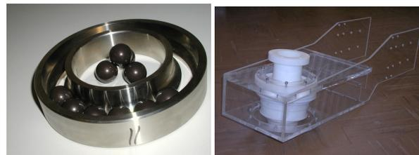
Figure 4: Left: View on the ceramic central ball bearing. Right: 1/1 plastic model of the cavity adapter lever arm.
