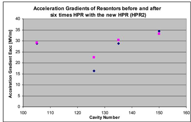
Figure 6: RF test results of nine cell cavities re treated with the new HPR system [Red=Eacc after re treatment; Blue=Eacc before treatment].
