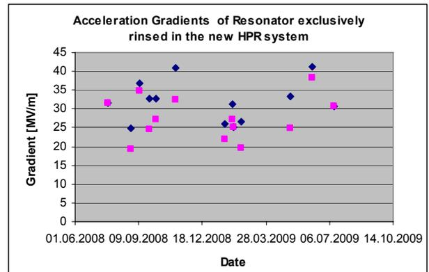
Figure 7: RF test results of nine cell cavities exclusively HP rinsed in the new HPR system [Blue=Maximum acceleration gradient; Red: radiation acceptance limit Eacc for FLASH [0.01mGy/min].
