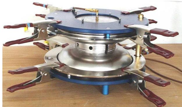
Figure 1: Simple RF-measurement device with clamped dumb-bell.
