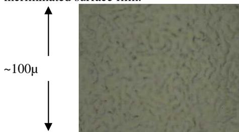
Figure 7: Typical features observed on samples after EP in aged mixture, with limited fluorine diffusion.
