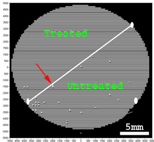
Figure 4: SFEM plot of field emitters on the surface of a BCP treated Nb coupon. Half of the coupon was treated with O<sub>2</sub> GCIB whereas the other half was not.
