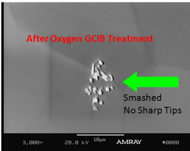
Figure 7: SEM image taken on an  $O_2$  GCIB treated Nb surface. The arrow indicates a potential emitter being “smashed” into pieces as if it were stepped on by a heavy Japanese sumo wrestler.
