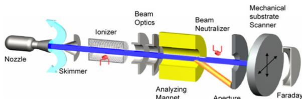
Figure 2: Schematic of working principal of GCIB.
