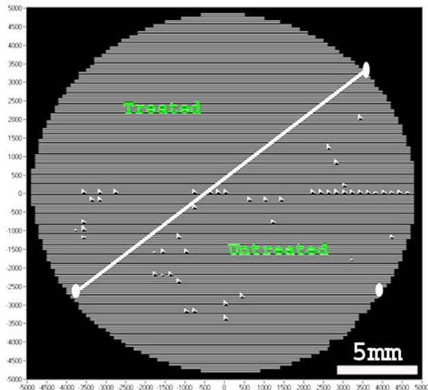
Figure 5: SFEM plot of field emitters on the surface of a BCP treated Nb coupon. Half of the coupon was treated with NF<sub>3</sub>+O<sub>2</sub> GCIB whereas the other half was not.
