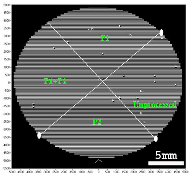
Figure 3: SFEM plot of field emitters on the surface of a BCP treated Nb coupon. The sample was masked into equal quadrants for treatments with Ar and/or O<sub>2</sub> GCIB or not treated as designated in the figure (see text for more details).
