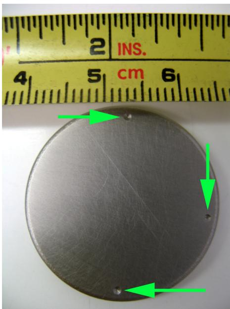
Figure 1: Standard Nb flat coupon used for the study described in this chapter. The arrows indicate the markings for coordinate identification.
