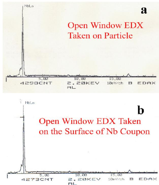
Figure 9: EDX spectra taken on a) one of the particle shown in Fig. 8, b) on the surface of the Nb sample.
