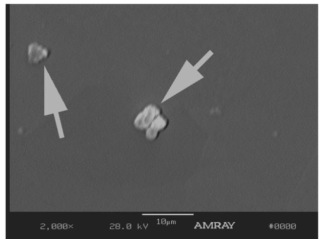
Figure 6: SEM image taken on an O<sub>2</sub> GCIB treated Nb surface. Two potential emitters as indicated by the arrows were suppressed by the treatment via removing sharp edges and tips.
