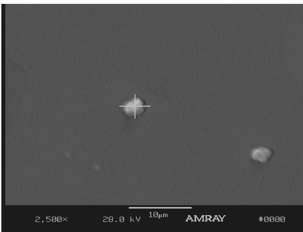
Figure 8: Close-up SEM image of two niobium oxide particles on the Nb surface treated by high energy  $NF_3+O_2$  GCIB. The two niobium oxide particles appeared to have smooth surfaces and to be embedded into the surface of the Nb coupon.
