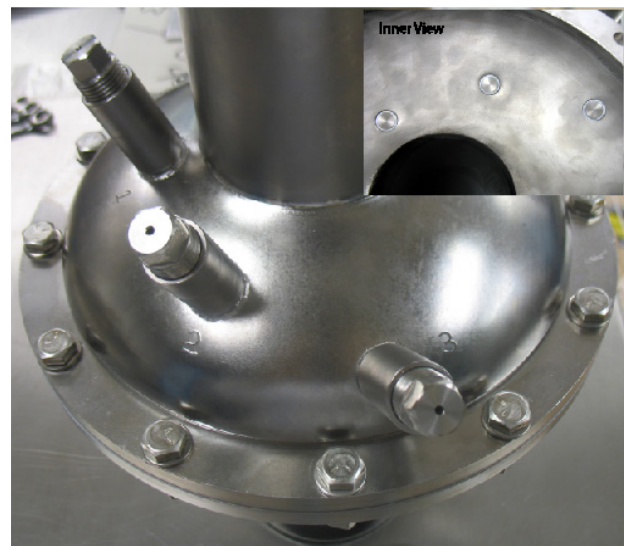
Figure 1: Demountable cavity for BEP study.
