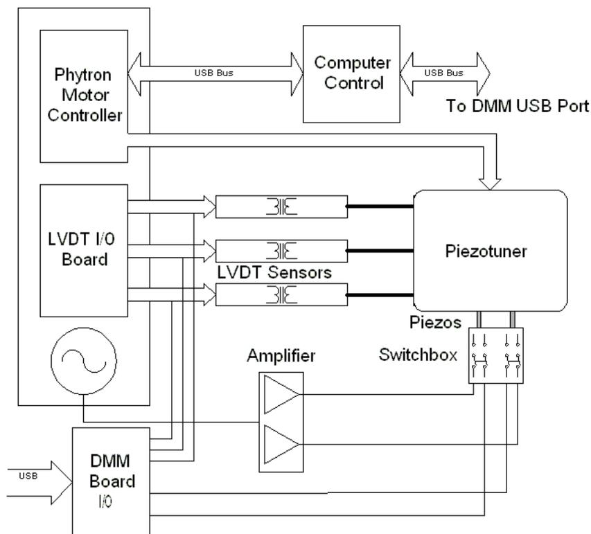
Figure 4: Block Diagram of the tuner test device.
