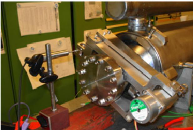
Figure 5: Piezo-tuner installed on C26 cavity at DESY.
