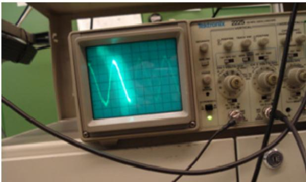
Figure 8: Cavity longitudinal displacement as seen by LVDT sensor: checking its amplitude and linearity is possible to check fast tuning capabilities.
