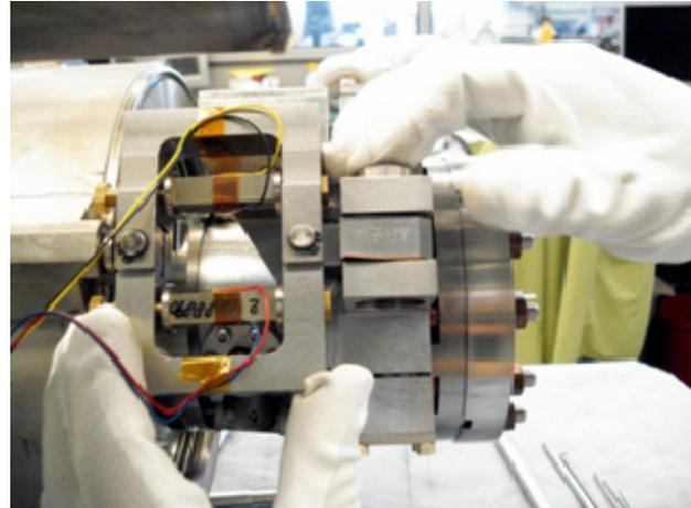
Figure 2: Piezo frame installation on the tuner.
