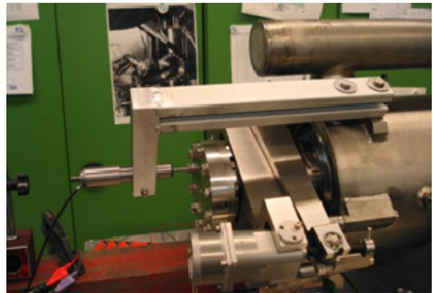
Figure 6: Sensor frame fixed to the two reference M8 holes on the cavity helium tank.
