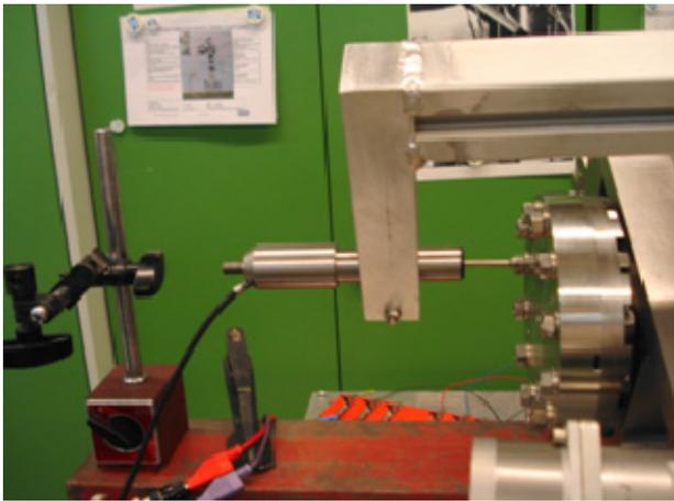
Figure 3: LVDT sensor installed in its frame.
