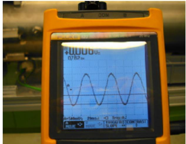
Figure 7: Signal coming from the piezo used as sensor: right polarity and good coupling are shown.
