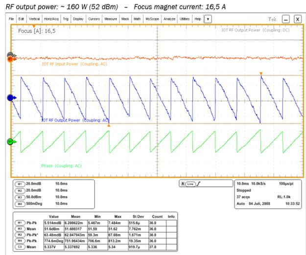
Figure 12: Typical time structure of the observed instability (IOT RF output power near 51 dBm, Focus current: 16,5 A). Green curve is the phase difference between IOT RF input and IOT RF output with 0,5 Deg/Div. Red curve is the AC component of the IOT RF input power with 0,02 dB/Div. Blue curve is the AC component of the IOT RF output power with 0,02 dB/Div. Grey curve is the DC component of the IOT RF output power with 50 dBm/Div.
