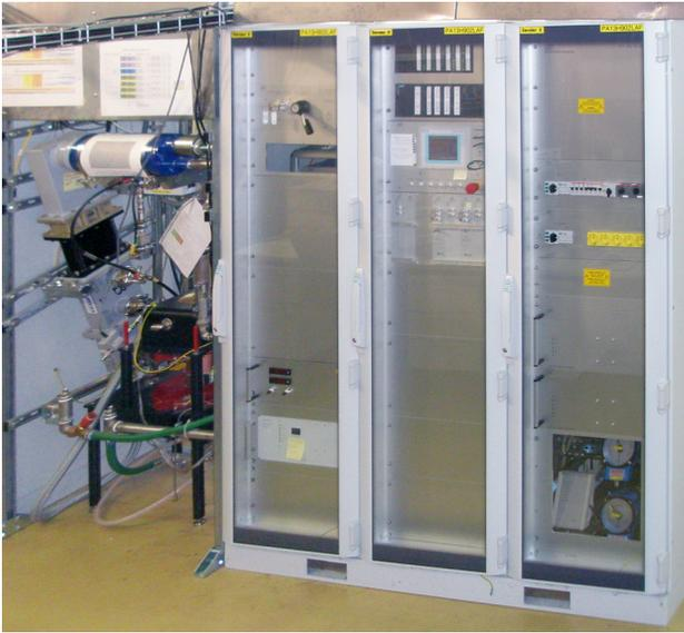
Figure 13: Three cabinets containing operating panel, interlock, all power supplies and the mains distribution. On the left the 1,3 GHz CPI IOT CHK5-1320W operating at a dummy load.
