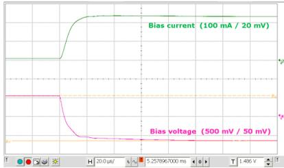
Figure 9: Cable resonances damped with a 5 Ohm series resistor and additional 1 $\mu$ F foil capacitor integrated into the tube socket. Step response measured with 20,0  $\mu$ s/Div at the tube socket.
