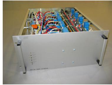
Figure 15: One of the two 20 kW driver units of the switching power supply of the beam voltage.
