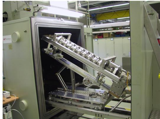
Figure 4: Electron beam welding plant at DESY, prepared with cavity for welding.
