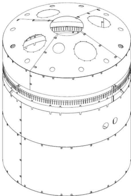
Figure 2: Magnetic Shield.
