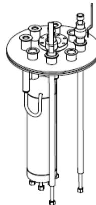
Figure 3: LN2 Phase Separator.
