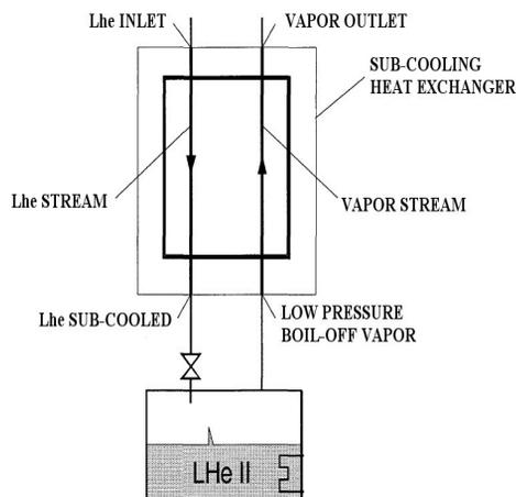
Figure 5: Heat exchanger flow schematic.
