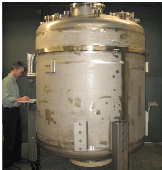
Figure 1: SRF Test Cryostat.
