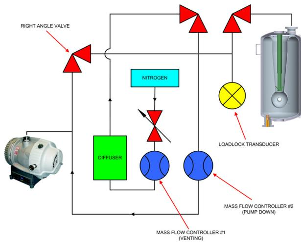
Figure 1: "Up-to-air" system schematic.
