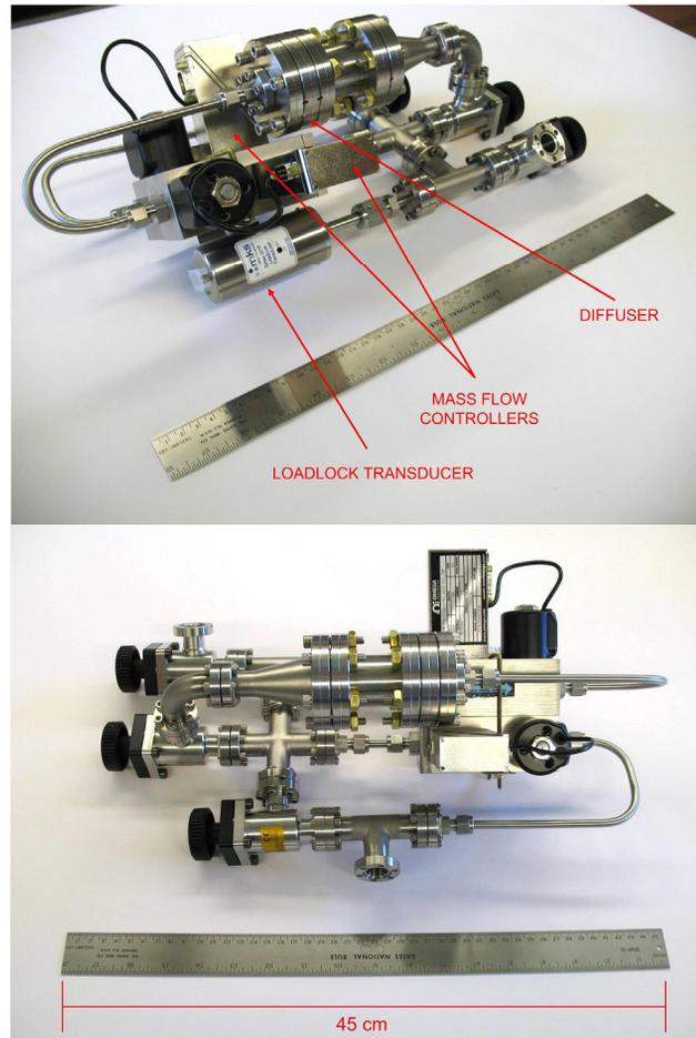
Figure 4: Assembled "up-to-air" system.
