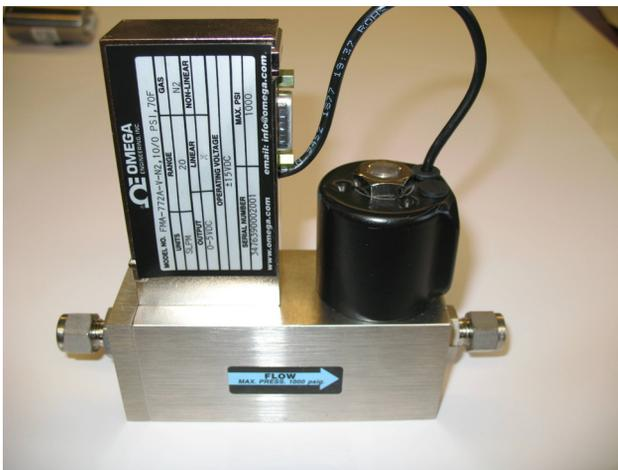
Figure 3: Omega Model #FMA-772A-V mass flow controller
