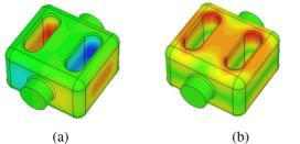
Figure 10: Surface (a) electric and (b) magnetic field of 800 MHz crabbing cavity.
