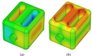
Figure 9: Surface (a) electric and (b) magnetic field of 400 MHz crabbing cavity.
