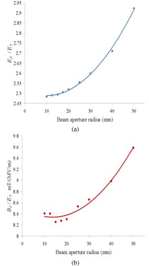
Figure 4: Change in peak surface (a) electric field and (b) magnetic field due to the change in beam aperture radius.
