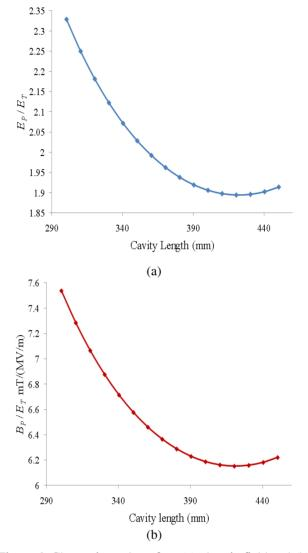
Figure 6: Change in peak surface (a) electric field and (b) magnetic field due to the change in cavity length.
