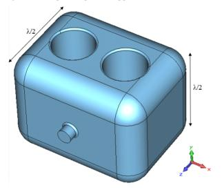
Figure 1: Parallel-bar structure.
