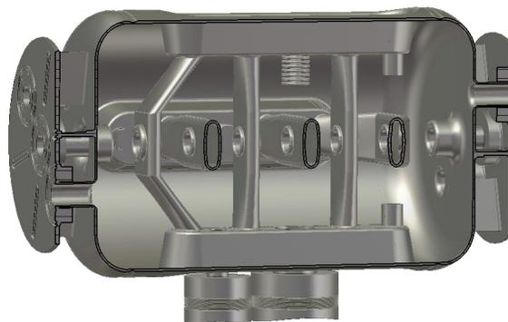
Figure 2: Design of the superconducting 7-cell CH-Cavity (325 MHz,  $\beta = 0.15$ )[6].
