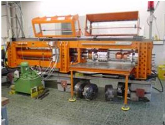
Figure 5: Hydro-forming apparatus for the production of seamless Niobium cavities
