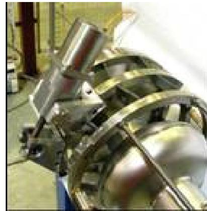
Figure 3: New tuning system for ILC type applications.
