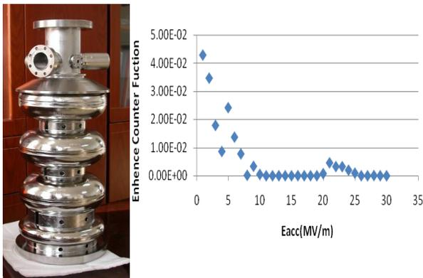
Figure 6: Simulation on multipacting of 3.5-cell cavity.
