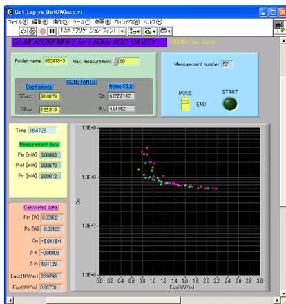
Figure 10: Vertical test result of SINAP single cell cavities.
