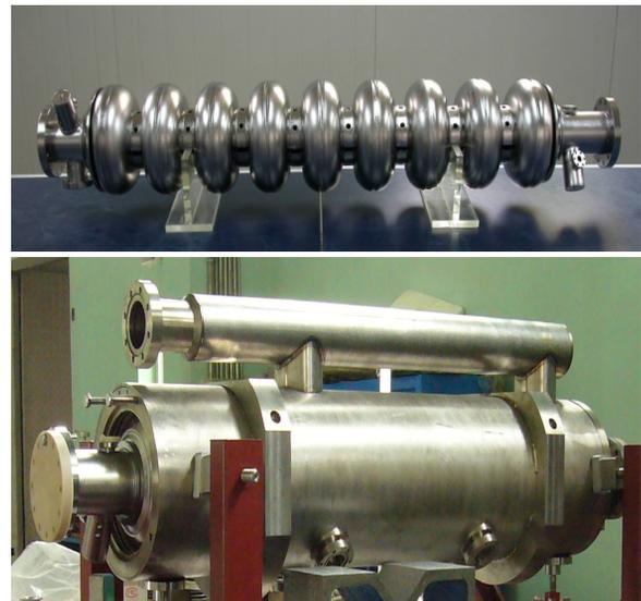
Figure 4: The 9-cell cavity of fine Nb grain with end groups in a Liquid He tank.
