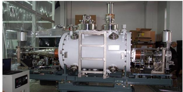
Figure 8: 500 MHz KEKB type SRF cavity for IHEP.
