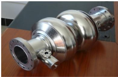
Figure 3: A 2-cell cavity of fine grain Nb with end-group.
