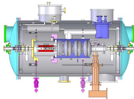
Figure 5: Schematic design of DC-SC Photo-injector.
