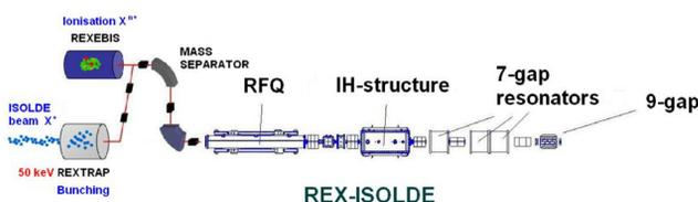
Figure 1: REX-ISOLDE present scheme.
