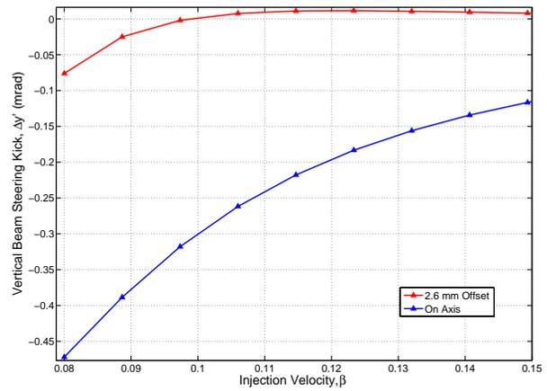
Figure 6: Divergence of the beam in case of a compensated (red) and not compensated (blue) case for a synchronous phase of -20 deg as a function of the incoming beam velocity.
