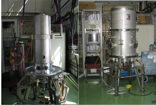
Figure 10: On the left the dummy cavity during mounting for the first sputtering. On the right the sputtering chamber closed
