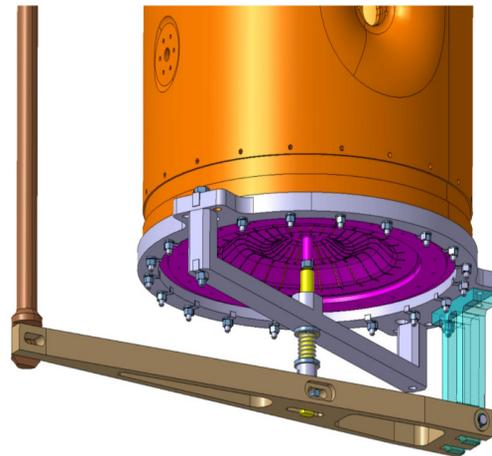
Figure 4: 3D view of the tuner with the lever actuator.
