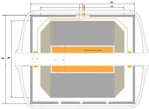
Figure 8: Solenoid schematics.
