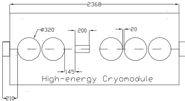
Figure 5: Schematics of the high energy cryomodule.
