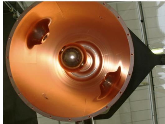
Figure 9: Cavity copper substrate towards final machining steps.
