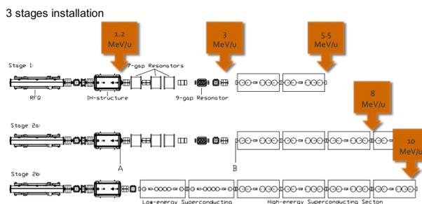
Figure 2: HIE-ISOLDE installation staging.
