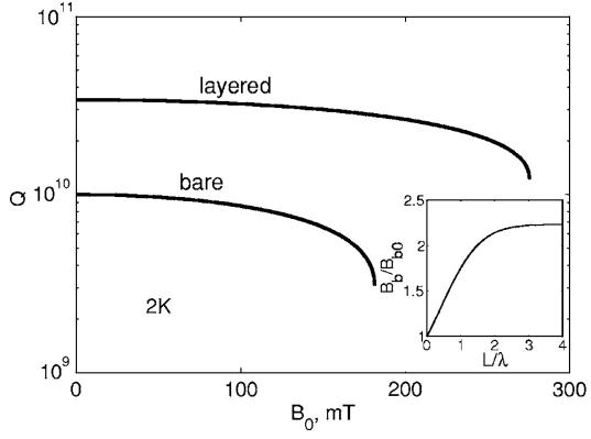
Shown in Fig. 3 is an example of *QB0 calculated* from Eqs. 11–14 for bare and 50 nm Nb3Sn clad Nb cavities at 2 K for =2, *Rb=20 n, R0=2 n at 2 K,* s=0.215, *D*=3 mm, h=5 kW/m2 K, =10 W/mK, and  $Q_0$  Nb=10<sup>10</sup>. In this case a 50 nm Nb3Sn overlayer more than triples *Q at* low field and increases *Bb* from 180 mT to 280 mT,
