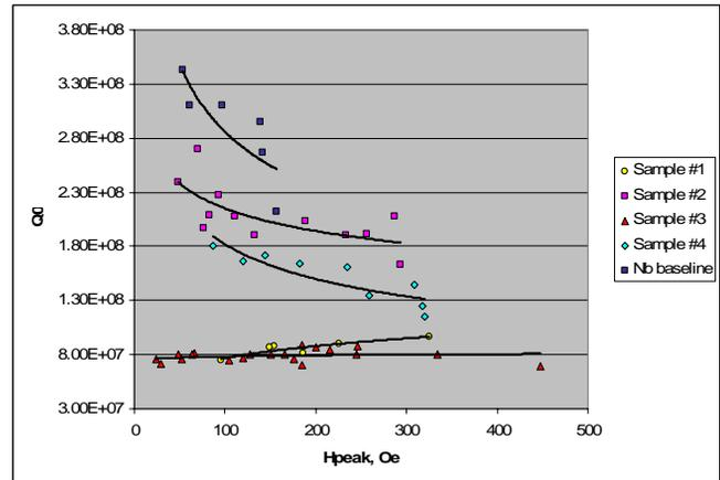
Figure 5: Q<sub>0</sub> versus peak magnetic field for different Nb/Cu end plates and a bulk Nb end plate.
