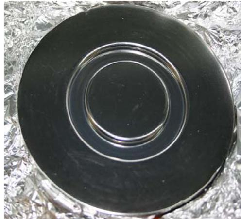
Figure 1: Nb-coated copper plate.
