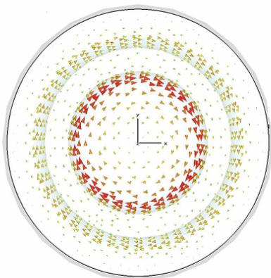
Figure 4: Currents at the bottom plate surface when the cavity is operated in TE<sub>011</sub> mode. Red arrows correspond to a larger current – high magnetic field region.
