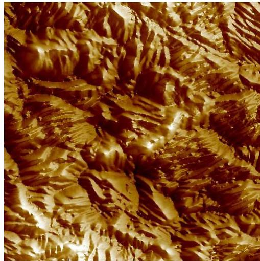
Figure 2: Atomic force microscope picture of the sample surface ( $2 \times 2 \mu\text{m}$  area). The surface roughness is about 400 nm as compared to EP bulk Nb (200 nm) and BCP bulk ( $2 \mu\text{m}$ ).
