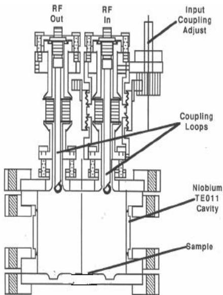
Figure 3: TE cavity schematic diagram.
