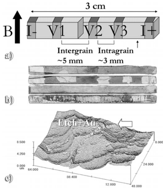
Figure 2: a) Schematic description of resistivity sample with b) images of each side of the actual sample. In c) we show a Laser Scanning Confocal Microscope image of the 1 μm thick Au contact layer.
