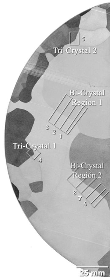
Figure 1. Overview of as-received ingot slice showing bi- and tri-crystal regions used for this series of experiments.
