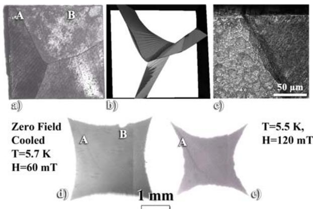
Figure 6: Tri-crystal #4 a) with 3D model b) and a height map of the top left hand grain boundary showing a  $13 \mu\text{m}$  step. A typical "rooftop" magneto-optical image (d) is obtained at  $T=5.5$  K,  $H=120$  mT. In d) and e) a faint line, marked “A” indicating a current inflection is observed and in d) an edge notch, marked “B”, which does not extend into the sample with increasing field (e).
