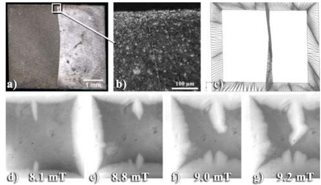
Figure 3: Bi-Crystal #1 a) with b) a height map detail from the area indicated, showing sub 5 μm topography at the grain boundary and c) a 3D model of the bi-crystal. A series of MO images, d)-g), at increasing field (T=5.6 K ZFC), shows premature flux penetration starting at a field of only 8.1 mT,  $\ll H_{c1}$ .
