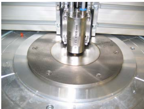
Fig. 1 SNS Eddy current scanner setup
