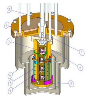
Figure 5: CAD model of new Fermilab 3R measurement insert. -1- sample, -2- pogo-pin, -3- helium heating channel, -4- G10 sample-holder, -5- sample insert insulating vacuum, -6- removable sample insert cover, -7- liquid helium supply, -8- support, -9- top flange;
