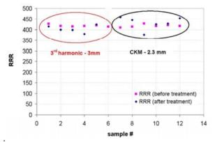
Figure 2: RRR test results on Nb for the FNAL 3<sup>rd</sup> harmonic and transverse deflecting (CKM) cavities, as received and after a complete standard surface treatment for cavities, including several cleaning, rinsing and etching steps as well as a high temperature anneal.
