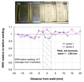
Figure 3: Top: Welding test fixture top after welding. The samples plates are clamped between Al plates Bottom:  $3^{rd}$  harmonic batch-1 weld series results (normalized to average RRR before welding, ~417). The grey region represents the weld.
