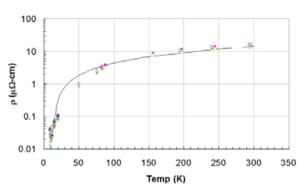
Figure 1: Electrical resistivity vs temperature as measured on 12 samples. Also shown: a simple fit (Eq. 1).
