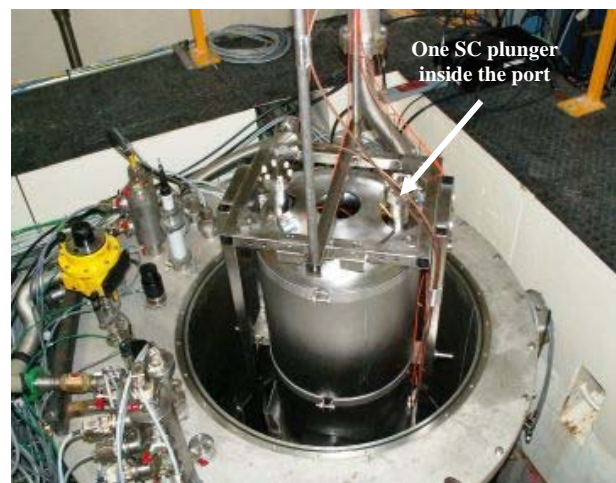
Figure 3: Beta 0.12 QWR before the test with a SC plunger in one of the top port.
