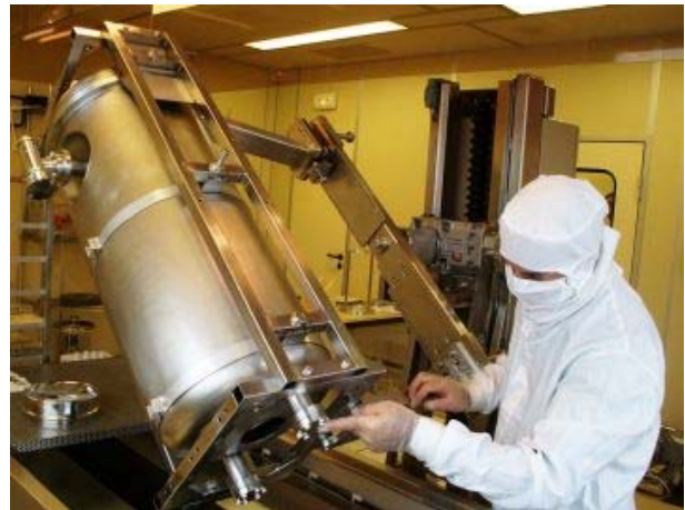
Figure 2: Beta 0.12 QWR inside the clean room before the High Pressure Rinsing process.
