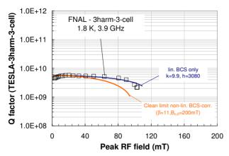
Figure 8: Comparison of measured quality factor of a Fermilab 3<sup>rd</sup> harmonic (3.9 GHz) 3-cell cavity to model predictions. Experimental data were obtained at 1.8 K. There are no after baking data.
