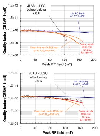
Figure 5: Comparison of measured and predicted quality factor of a JLAB low loss, single cell CEBAF cavity (LLSC, 1.5 GHz) before (top) and after (bottom) baking. Experimental data were obtained at 2.0 K.
