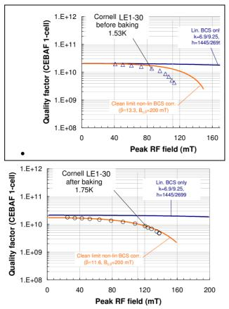
Figure 3: Comparison of measured and predicted quality factor of a Cornell University single cell CEBAF cavity (LE1-30) before (top) and after (bottom) baking. Experimental data were obtained at 1.53 K before and 1.75 K after baking. The bath temperature increased by  $\cong$ 50 mK during the test.
