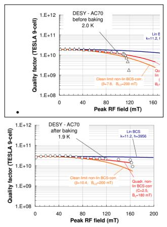
Figure 4: Comparison of measured and predicted quality factor of a DESY 9-cell TESLA cavity (AC70) before (top) and after (bottom) baking. Experimental data were obtained at  $\sim$ 1.9 K. The cavity was electro-polished.
