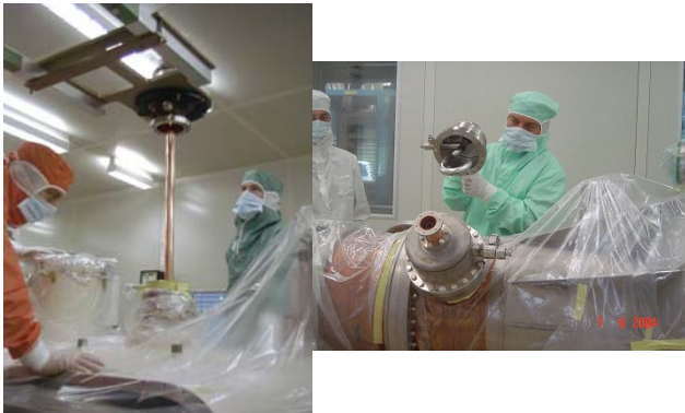
Figure 5 : IPC and HOM coupler assembling inside the CERN clean room
