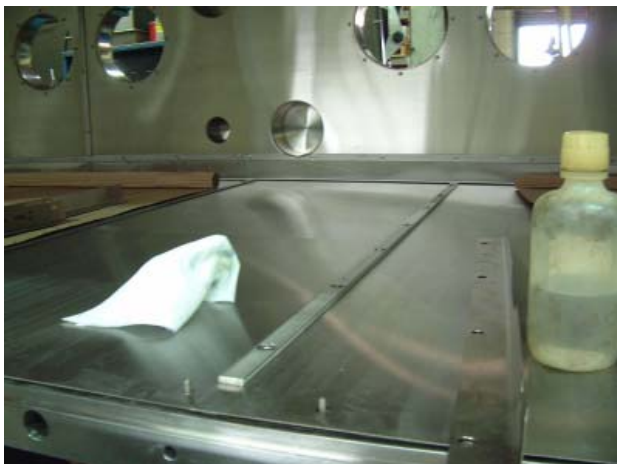
Figure 3: Magnetic shield panels with SS batten strips.
