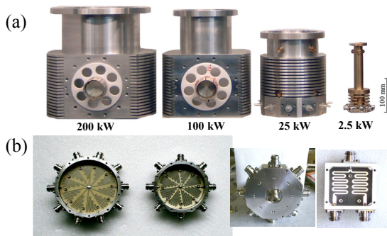
Figure 8 : Power combiners (a) and splitters (b)
