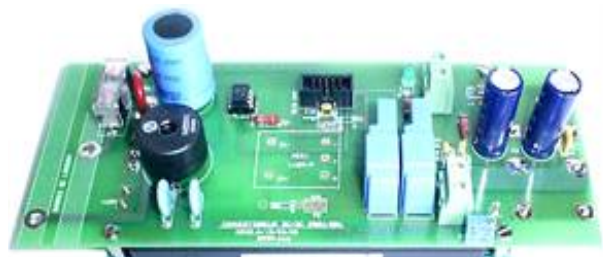
Figure 2: DC/DC converter board
