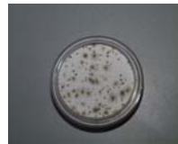
Figure 9: Analysis of UPW in the sump of the HP rinse stand
