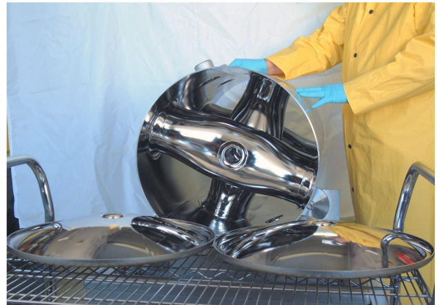
Figure 4: Electropolished subassemblies of the beta=0.63 triple-spoke resonator after final chemical processing at ANL.
