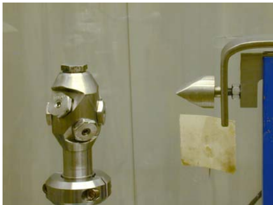
Fig. 1 Load cell equipped with a 30° wedge for angular dependence measurement of water jet force and profile.
