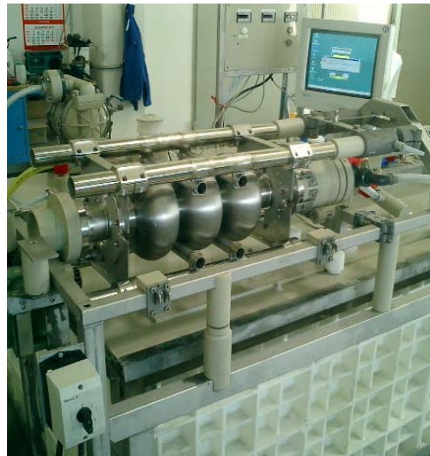
Figure 1: Setup for electropolishing
