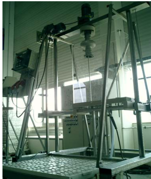
Figure 2: Setup to rinse cavity with high pressure pure water.
