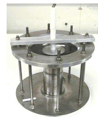
(c) Beam-tube welded half-cell cavity assembly
